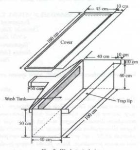
Fig. 2. Wash trap design
